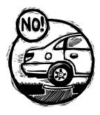
**DON'T** drive your vehicle or any heavy machinery over the lid or surface of your tank or cover buried components of your system. If there is a chance of vehicular traffic over your system, construct a barrier or plant rows of shrubs that would block this traffic.
